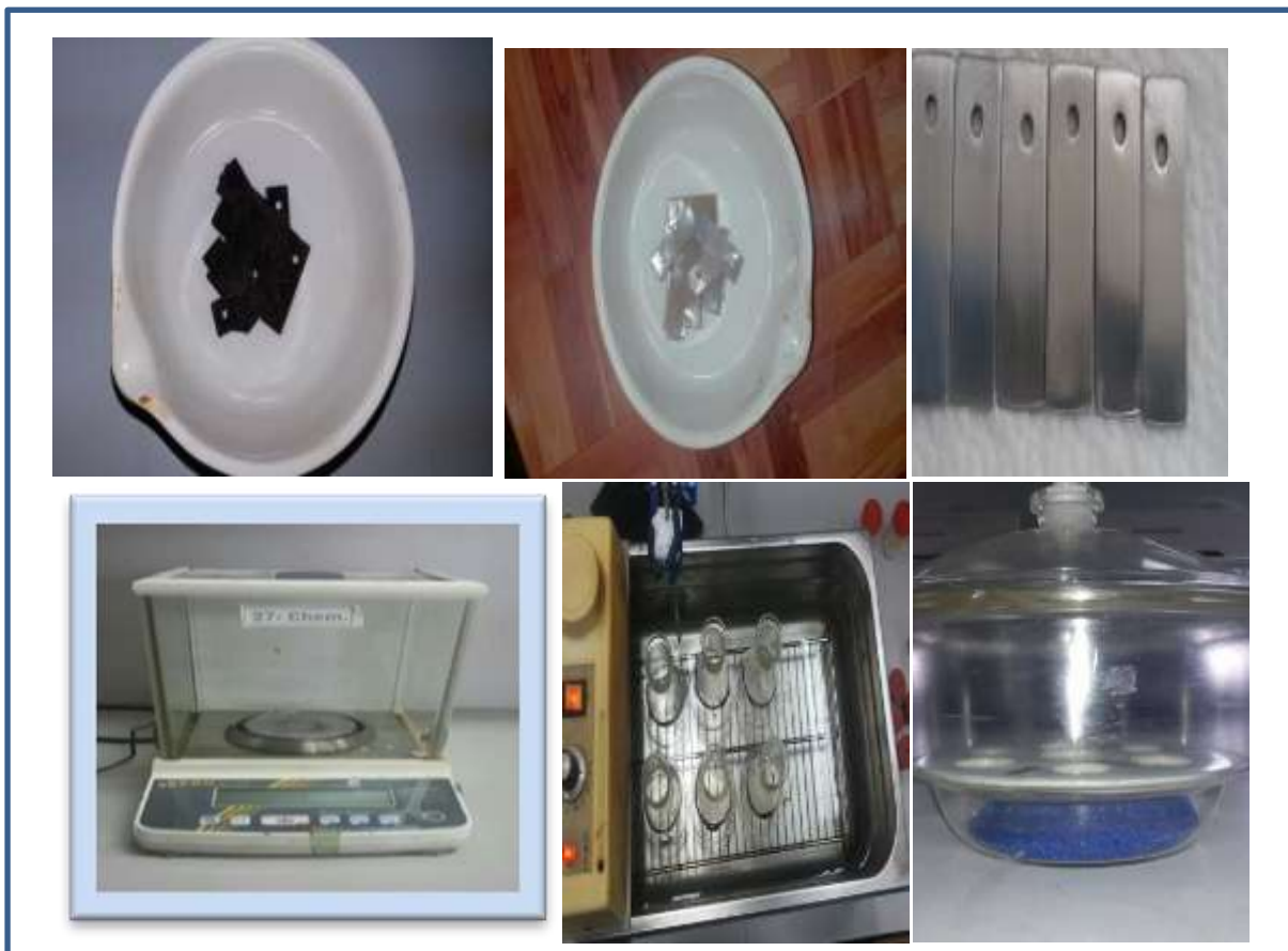
Figure(3.2) The preparation steps of the low carbon steel samples
