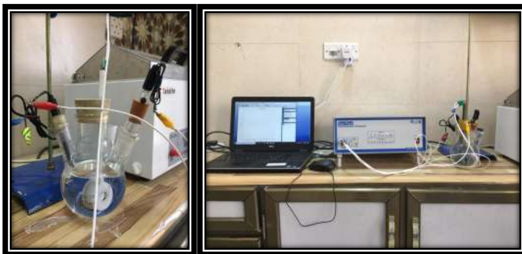
Figure (3.7) The Corrosion Cell used.
