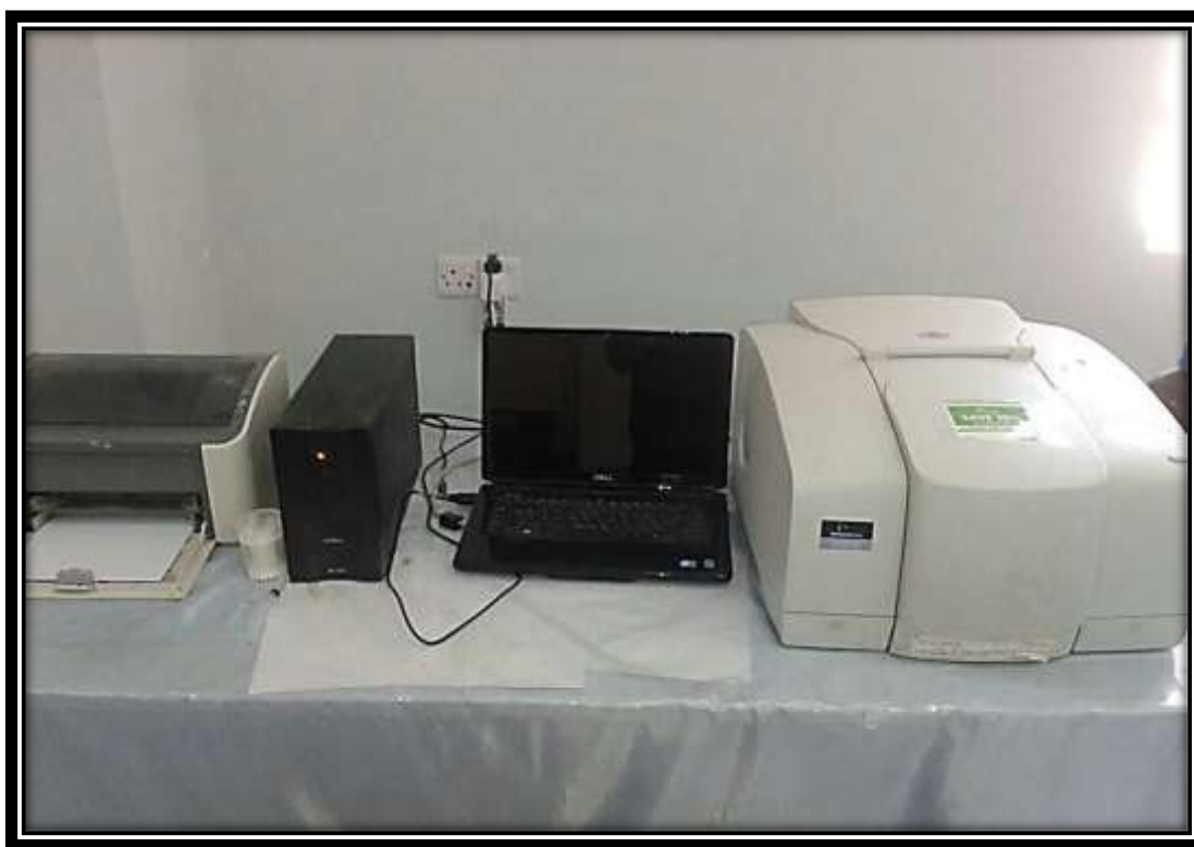
Figure (3.5) FTIR Infrared spectrophotometer used.
