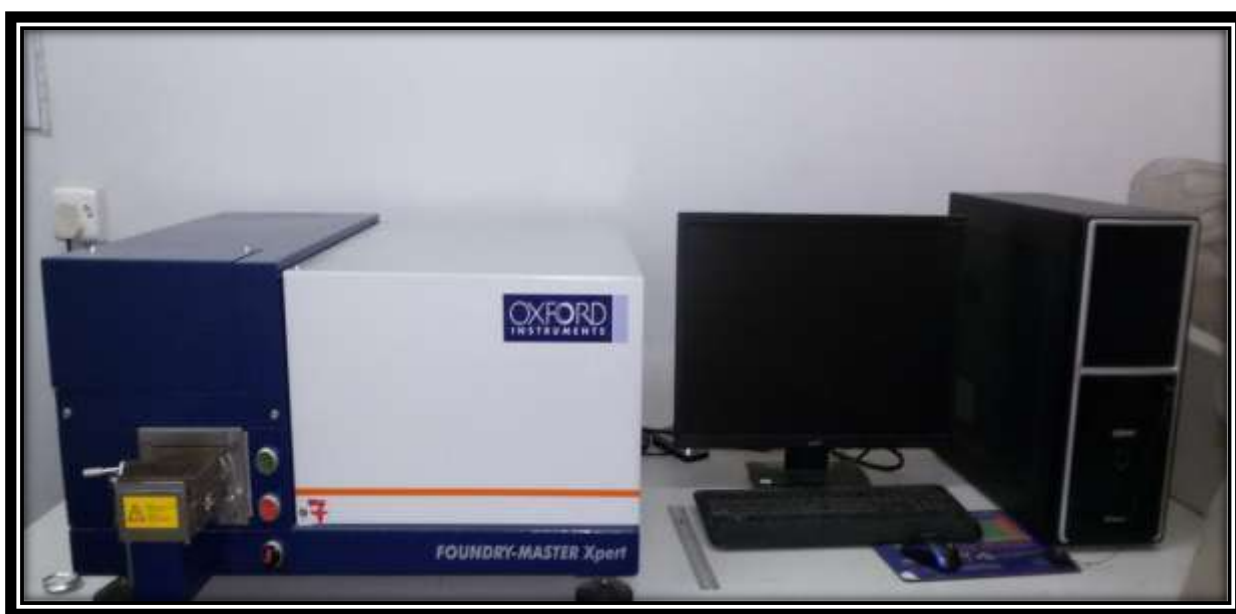
Figure (3.6) Optical Emission Spectrometer(OES) used.
